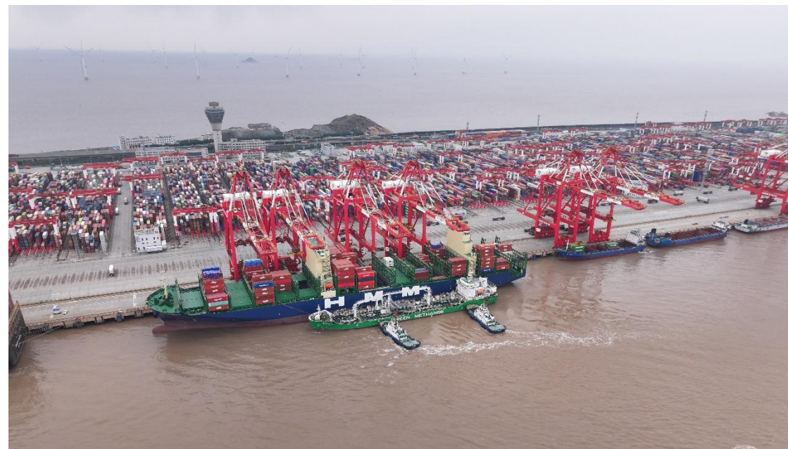
国产绿色甲醇同步作业加注 Domestic Green Methanol SIMOPS Bunkering
